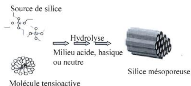
Fig.1. The MCM-41 formation mechanism proposed by Beck et al. [15]
